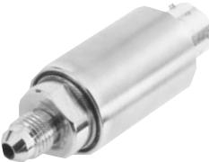
Providing long-term stability and reliability, the OMEGADYNE™ PX1200 Sputtered Gage High Output Pressure Transducer is a highly accurate thin film transducer. The thermal sensitivity error band performance is typically better than 0.25% within any 50°F temperature band.
